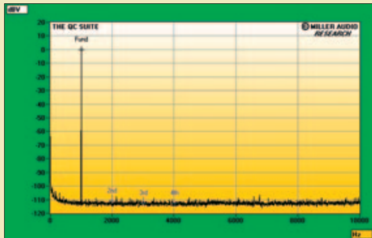
Fig.6 Halcro dm58, spectrum of 1kHz sinewave, DC-10kHz, at 200W into 8 ohms (linear frequency scale).
