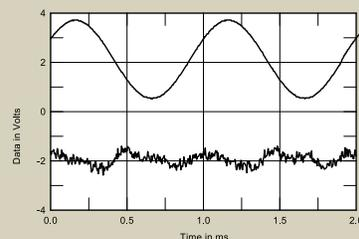
Fig.5 Halcro dm38, 1kHz waveform at 1W into 8 ohms (top), 0.002% THD+N; distortion and noise waveform with fundamental notched out (bottom, not to scale).
