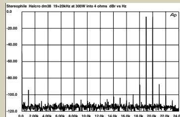
Fig.10 Halcro dm38, HF intermodulation spectrum, DC–24kHz, 19+20kHz at 300W peak into 4 ohms (linear frequency scale).
