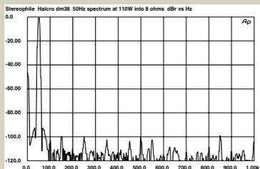
Fig.8 Halcro dm38, spectrum of 50Hz sinewave, DC–1kHz, at 110W into 8 ohms (linear frequency scale).
