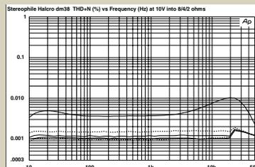
Fig.4 Halcro dm38, THD+N (%) vs frequency at 10V into (from bottom to top): 8 ohms, 4 ohms, 2 ohms (right channel dashed).
