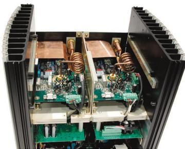
The densely packed upper module carries the input circuitry and the I/O hardware.
