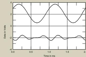
Fig.6 Halcro dm38, 1kHz waveform at 61W into 8 ohms (top), 0.0015% THD+N; distortion and noise waveform with fundamental notched out (bottom, not to scale).
