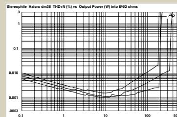
Fig.3 Halcro dm38, distortion (%) vs 1kHz continuous output power into (from bottom to top at 100W): 8 ohms, 4 ohms, 2 ohms.
