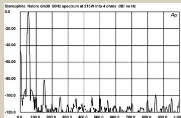
Fig.9 Halcro dm38, spectrum of 50Hz sinewave, DC–1kHz, at 215W into 4 ohms (linear frequency scale).
