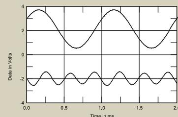
Fig.7 Halcro dm38, 1kHz waveform at 120W into 4 ohms (top), 0.0055% THD+N; distortion and noise waveform with fundamental notched out (bottom, not to scale).
