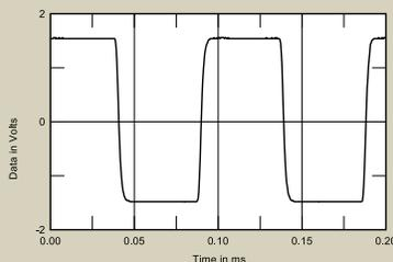
Fig.2 Halcro dm38, small-signal 10kHz squarewave into 8 ohms.
