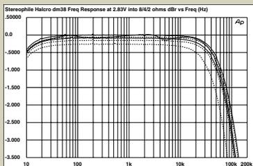
Fig.1 Halcro dm38, frequency response at 2.83V into (from top to bottom at 2kHz): simulated loudspeaker load, 8 ohms, 4 ohms, 2 ohms (0.5dB/vertical div., right channel dashed).
