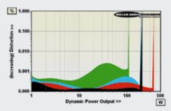
ABOVE: Dynamic power output versus distortion into 80hm (black trace), 40hm (red), 20hm (blue) and 10hm (green) speaker loads. Max. current is 10.4A
