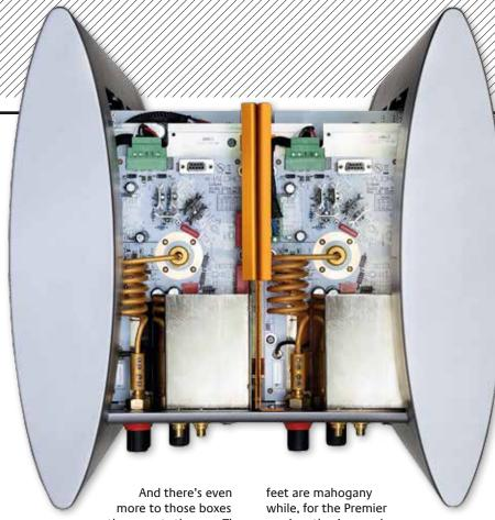
than meets the eye. The lower, larger housing contains the power supply, compete with IEC mains input and master power switch, while the upper section [pic, above] houses the input and output amplifier stages, each shielded from the others in more aluminium and copper. Every part of the amplifier's structure is hand-sprayed with multiple layers of aerospace-grade paint, and the whole enterprise sits on feet hand-carved from wood by a local luthier – or guitar-maker
