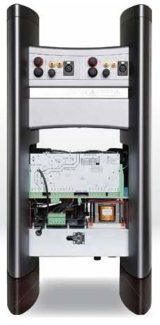
THERE ARE THREE INPUT MODES: UNBALANCED (22-KOHM IMPEDANCE); BALANCED (22-KOHM + 22-KOHM); AND MINIMAL PATH (660-OHM)
